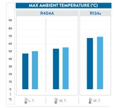
H.T.: evap. T. +5°C; cond. T. +50°C M.T.: evap. T. -10°C; cond. T. +45°C L.T.: evap. T. -35°C; cond. T. +40°C
